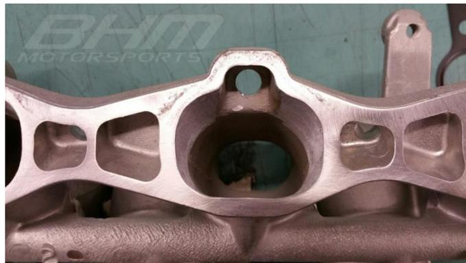
This shows the modified lower flange of the 3.5L 6G74 intake manifold. Here you can see the material to be removed for a MIVEC port match of the lower intake manifold to the 3.8L MIVEC cylinder heads.
